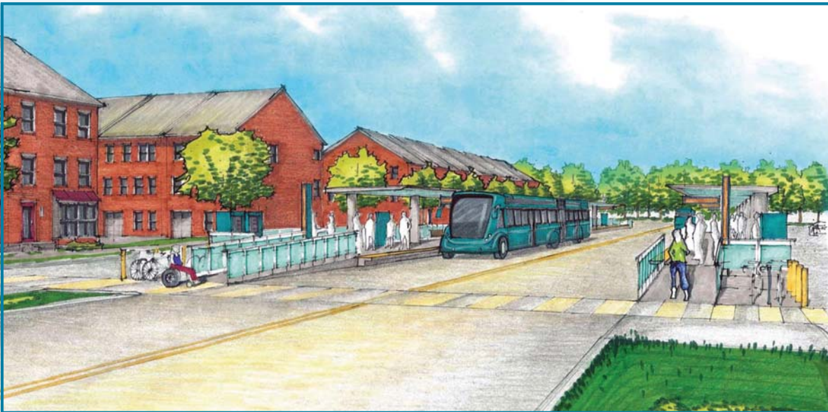
Side Platform Station
