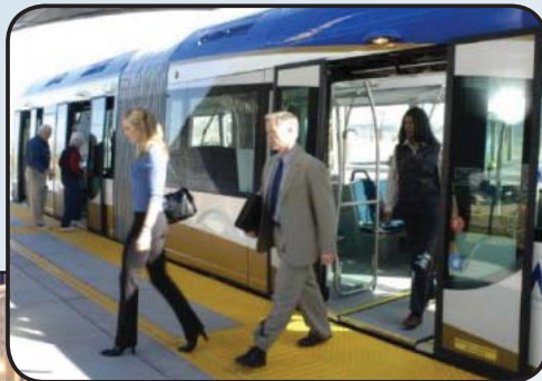
Las Vegas MAX (RTCSNV) features a low floor with level boarding platform
