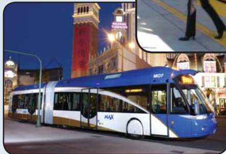
Las Vegas MAX (RTCSNV) features a low floor with level boarding platform
